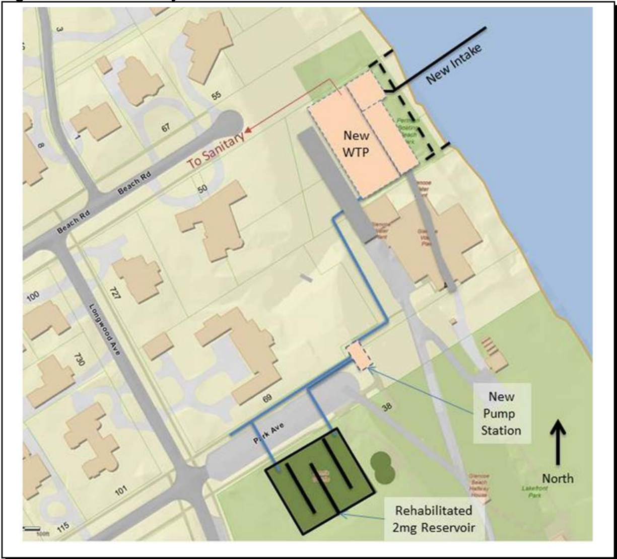
Figure 5.04-3 Preliminary Site Plan–North Lakefront WTP Location
